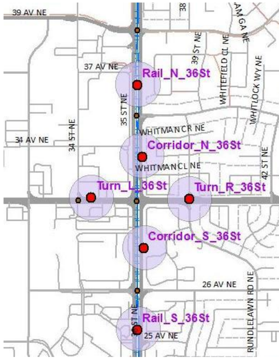
Figure 3: Bluetooth detector locations (red dots) and 100m detection radii (purple translucent circles)
